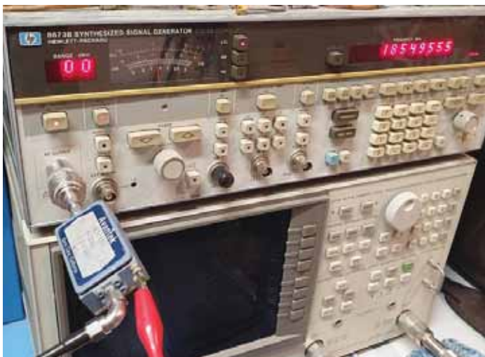
Figure 11 — The microwave signal source and amplifier.
