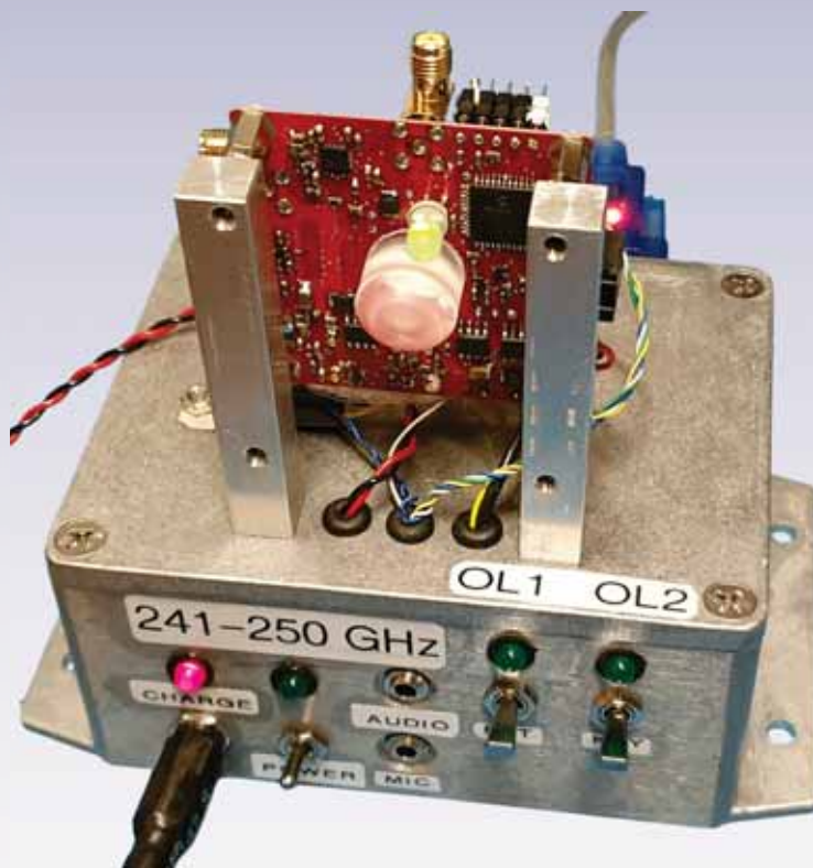
Beacon assembly for the 241 – 250 GHz Transverter.
